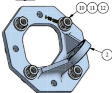
1. Align holes of item 2 with 4 studs on back plane of the antenna (not shown).
